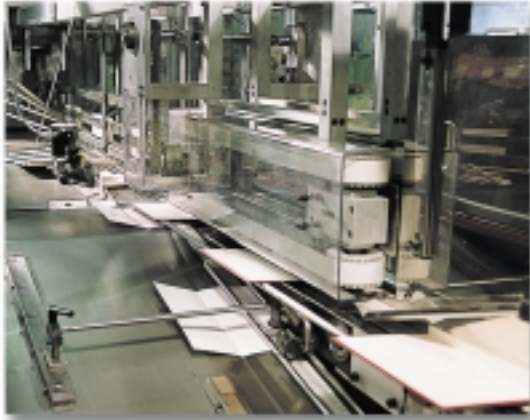
Paper feeding station adds the jackets automatically.
